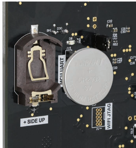
Figure 25. GBX Circuit Board Battery Replacement
