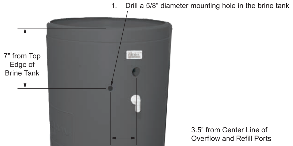
Figure 88. Brine valve float height.
