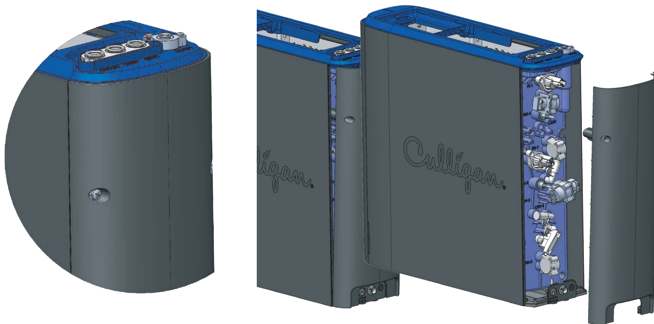
Figure 11. Rear Cover Removal
